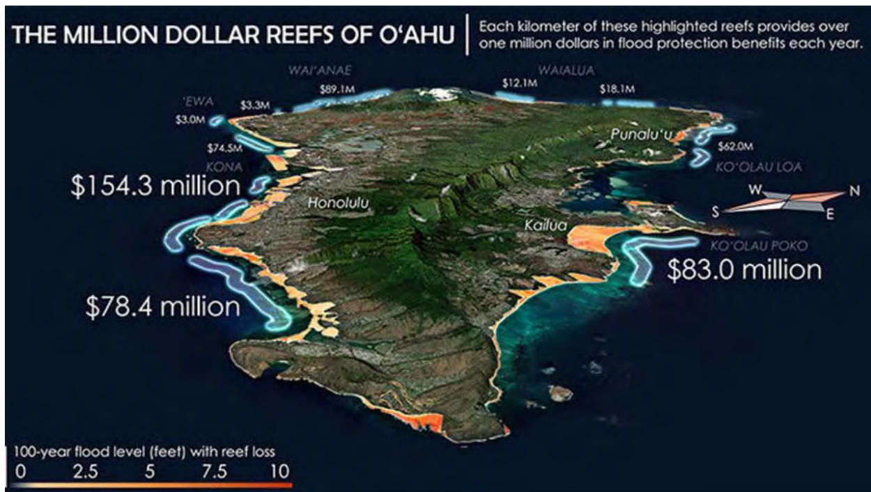
Figure 16. The highlighted reefs around O'ahu all provide greater than USD$1 million in expected flood reduction benefits per kilometer per year. The values in the figure are the sum of the annual expected benefits for reef sections that are several kilometers long (modified from Storlazzi et al., 2019; Reguero, 2021).
