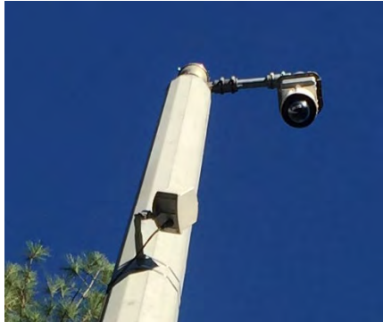
ROADWAY CCTV CAMERA AND TRAFFIC SENSOR (MDVS)
