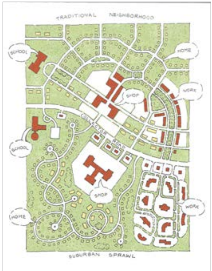
Figure 45: By offering more choices, a network of smaller streets provides greater capacity than a disconnected hierarchy of large streets.
